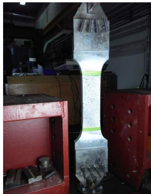
Figure 4 Tensile specimen geometry and loading arrangement
