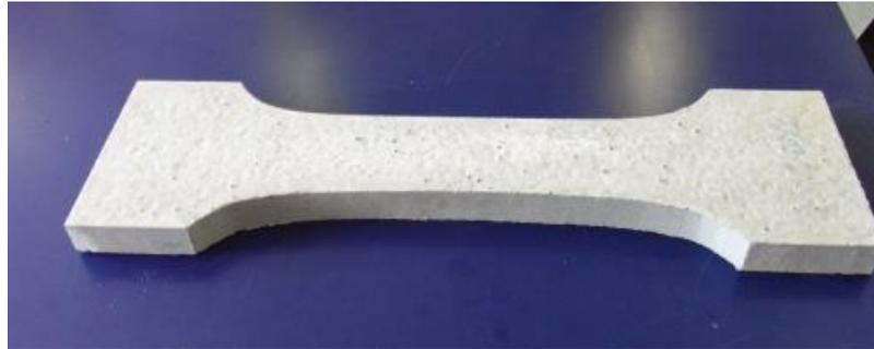
Figure3 Concrete tensile specimen
