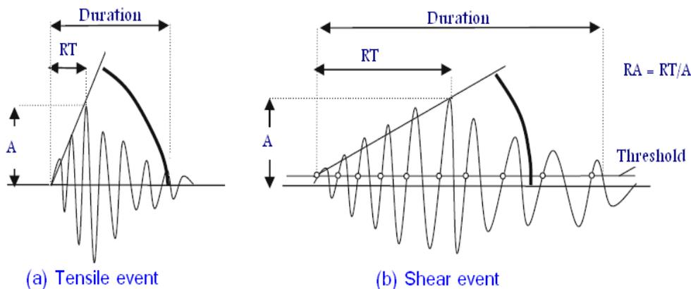
Figure 1 Typical waveforms (Soulioti et al 2009)
