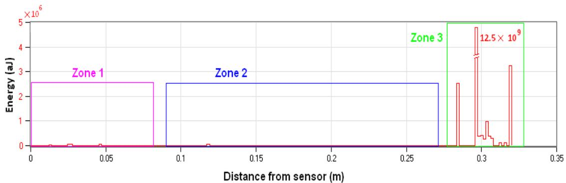
Figure 11 Absolute energy vs. liner location
