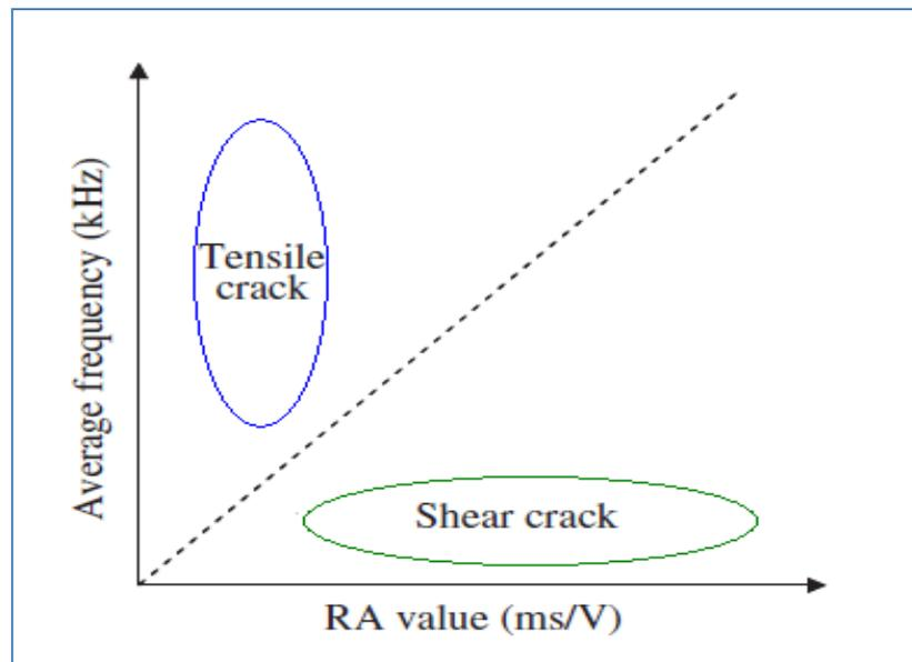
Figure 2 Crack classifications (Ohno and Ohtsu 2010)
