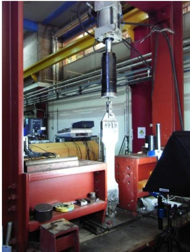
Figure 5 Photograph of concrete specimen in the test machine
