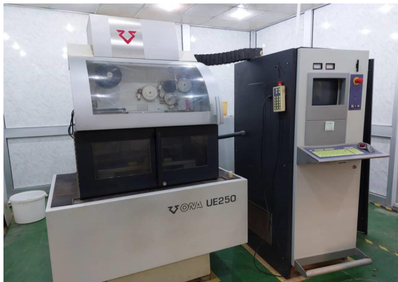
Fig. 2: ONA Electro-Erosion Machine ( Available at the Araian Gulf Oil Company Central Workshop, Ganfooda , Benghazi)
